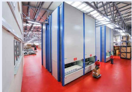
In some cases, warehouses with limited ceiling heights have constructed a vertical storage unit outside of the existing building, enclosed it and provided access to the unit through an existing exterior wall. This allows the benefits of the storage height without the restriction of the building ceiling – avoiding leasing an additional facility or a full building expansion.
