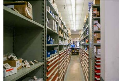
If you need to access product with a pallet jack, the aisle space increases to 4 to 5 feet wide. If product needs to be accessed with a forklift, it's far greater as you need to accommodate the length of the forklift plus an additional 12 inches of maneuvering space. A standard forklift can require 12 foot aisles – you can get this aisle space down to around 4 feet with a narrow aisle order picker.
