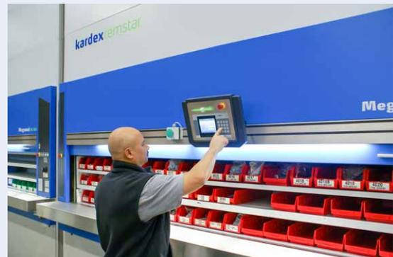
Consolidating all of the aisle space found in a typical shelving system into one access point recovers a considerable amount of floor space. This recovered floor space gives you room to expand operations internally, avoiding a costly facility move or expansion (not to mention eliminates the time workers spend walking and searching through shelving as all stored product is now delivered directly to the worker).
