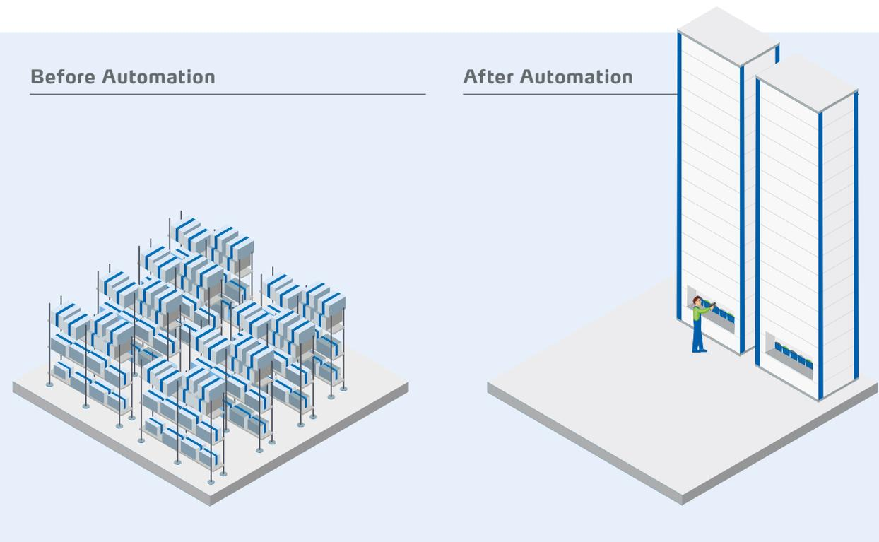
Implementing an automated solution immediately reduces the amount of square footage required to store items within static shelving and pallet rack in two ways: one, by utilizing previously unused overhead space, and two, by compressing items stored within the technology for greater storage capacity. This is because the volumetric efficiency of each automated technology is so much greater, shown below.
