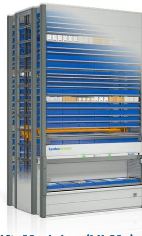
**Vertical Lift Modules (VLMs)** – An enclosed automated storage and retrieval system that incorporates two columns of trays with a central inserter/extractor that automatically locates and retrieves stored trays from both columns, then presents them to the operator at a waist-high pick window. These systems save up to 85% of floor space compared to static shelving and rack.
